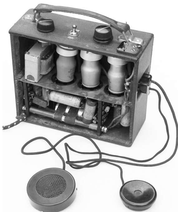
Figure 3-0: An early electronic hearing aid by the English company Amplivox with 3 vacuum tubes (made by Mullard). This table model (dimensions 19x18x7.5 cm) with external microphone dates from 1938. Tone switch (right) and volume wheel (left) are located on top. Mains cord for power supply (220V AC). Circuit diagram reconstructed by the author (resistor values in Ohms, capacitor values in Farad). Hearing aid from the historical collection of Beter Horen, Doesburg, the Netherlands. Photograph by the author.
