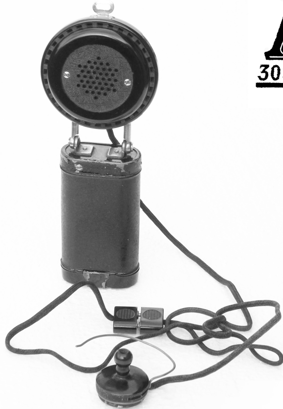
Figure 2-0: Early electric hearing aid with carbon microphone by Ardente, dating from around 1930. The volume can be set by a switch that is situated at the back of the microphone. The box below contains two 1.5 Volt batteries. Electrical diagram reconstructed by the author (resistor values in Ohms). Hearing aid from the historical collection of Beter Horen, Doesburg, the Netherlands. Photograph by the author.
